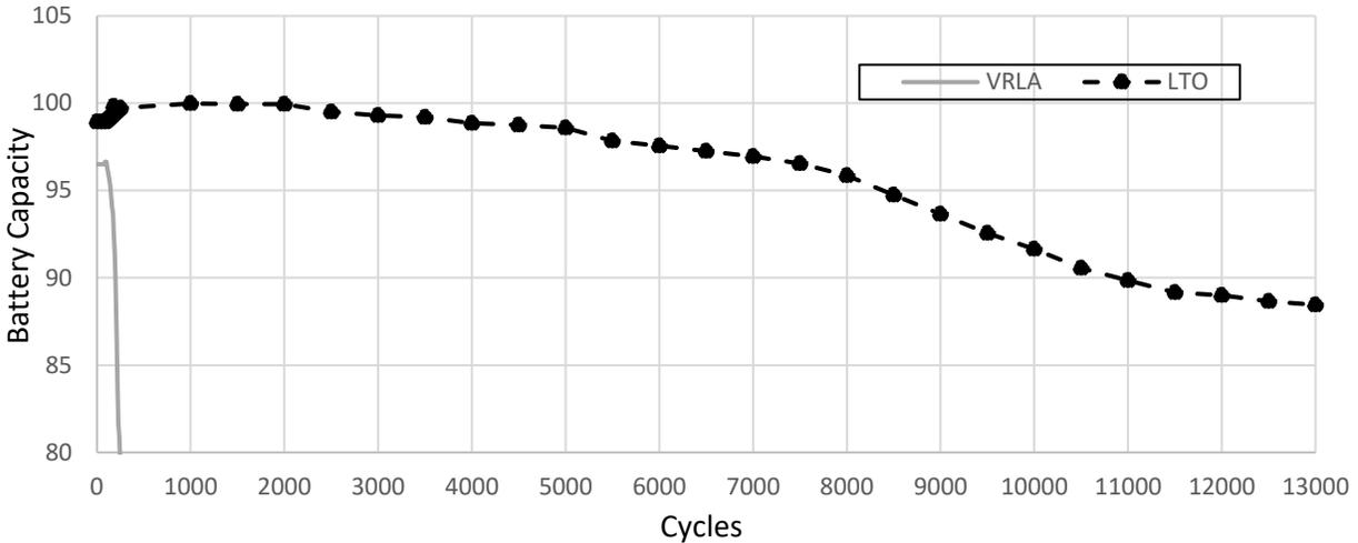
Figure 1: Life Cycle Comparison of LTO and VRLA\*\*
